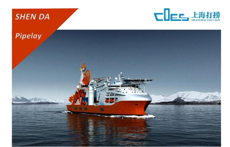
The SHEN DA is a DP Class 3 Vessel designed with a reel-lay system capable of rigid, flexible, umbilical and piggyback lay, maximum to water depths up to 3000m for worldwide operations.
